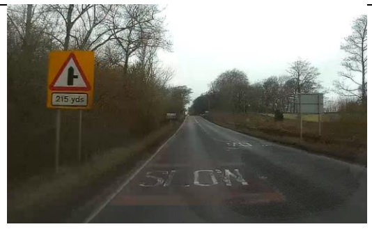
Photo 18 – Example of use of yellow backed junction warning sign with supplementary distance plate.
